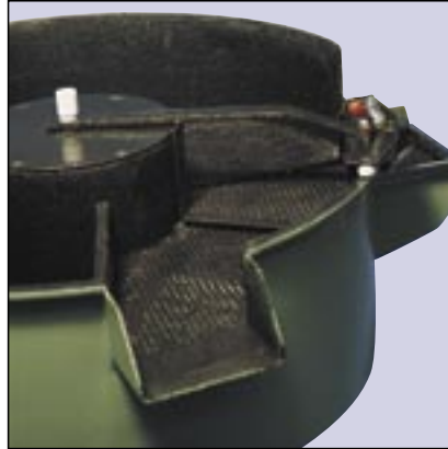
Polyurethane Spray Coating
