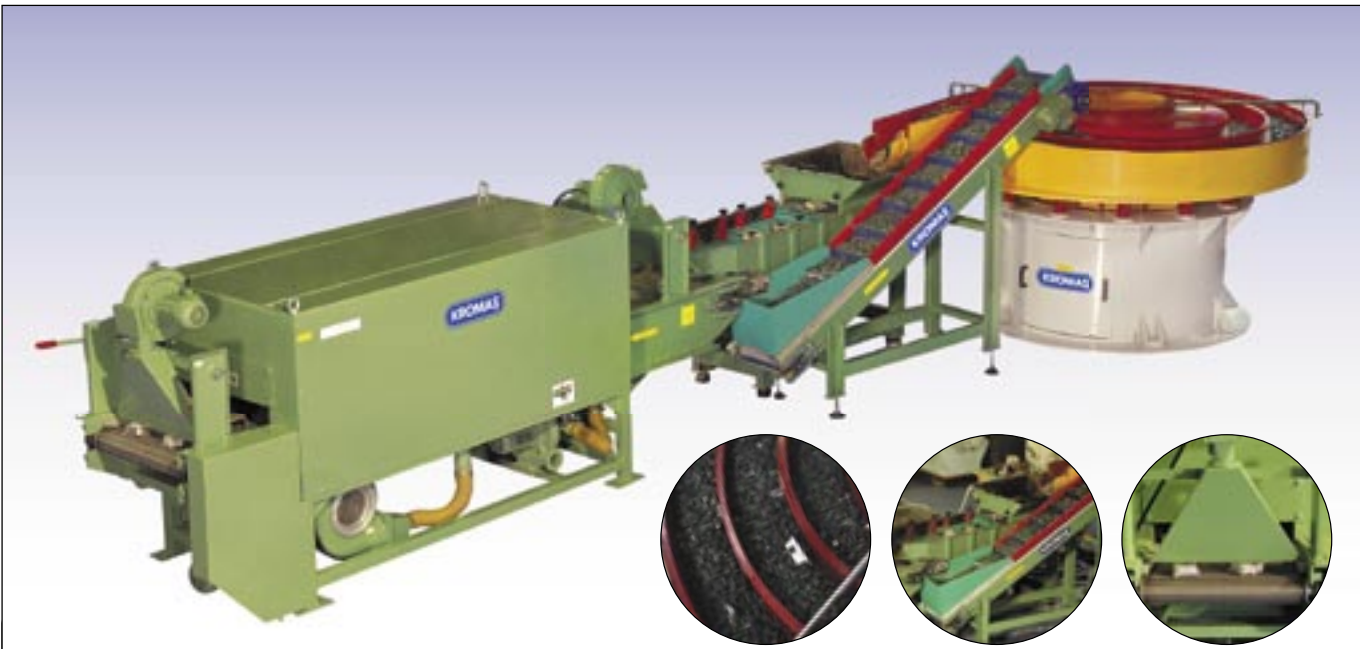
ATC 200 & TNL 4000 Spiral Continuous Finishing System & Tunnel Drying Machine
